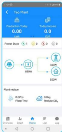
By pressing the Home button you can see how the electricity is distributed.
