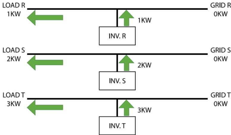
**Total Phase Power:** The inverter delivers the total power needed to match the total load on all phases equally. If on a certain phase the power delivered is greater than the load, the remaining power will be injected in grid; if it is less, then the difference will be supplied from the grid.
