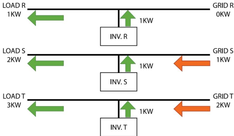
**Independent Phase Power (this option is available for hybrid inverters!):** The inverter tries to supply the required power on each phase to match each load, without taking power from the grid if possible.
