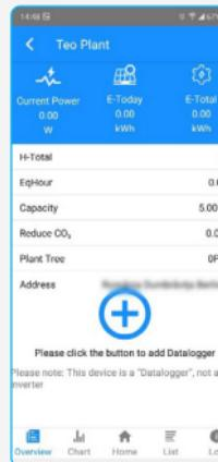
If the inverter has an attached Smart meter or CT, then the inverter serial number will be needed in the Overview screen.
