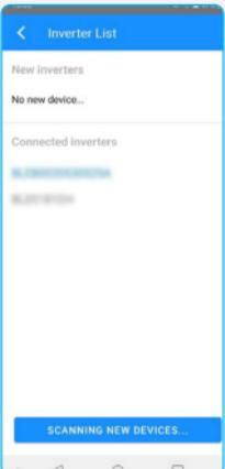
To successfully connect the inverter serial number needs to be added, by scanning or by manual adding and selecting the inverter's name from the available Bluetooth connections. (The Product serial number can be found on the side label attached to the inverter).
