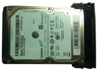
② Make sure the HDD metal surface is facing up and then put the HDD into the bracket
